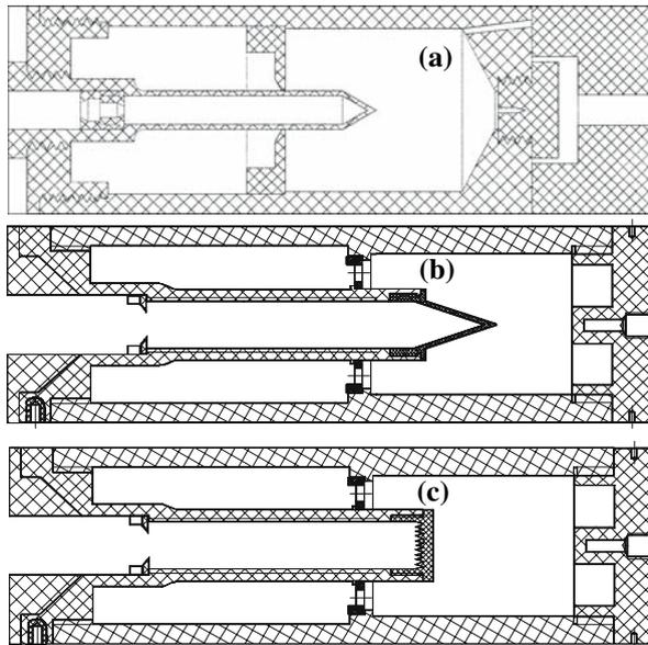
**Fig. 3** Designs of three graphite fixed-point blackbody cavities: (a) 6 mm diameter small cavity w/60° cone bottom, (b) 12 mm diameter cavity w/37° cone bottom, and (c) 12 mm diameter cavity w/v-groove bottom
