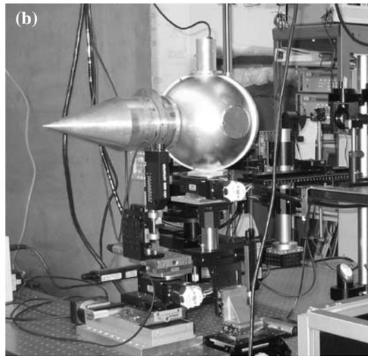
the port cover is placed onto the port. There are several ways to perform the reference measurements. For the measurements as described here, we are using a substitution mode. In this case, we separately characterize and correct for the sphere throughput change between measurements.
