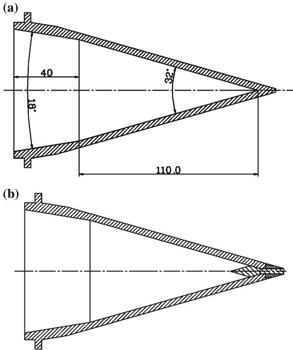
**Fig. 4** Designs for three blackbody cavities: (a) variable-temperature water-bath cavity and Ga fixed-point cavity with a straight cone bottom and (b) Ga fixed-point cavity with a combination straight and inverted cone bottom (dimensions in millimeter)
