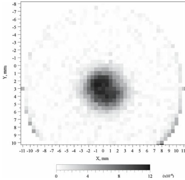
Fig. 10 Effective emissivity of cone cavity for water-bath blackbody: initial coating
