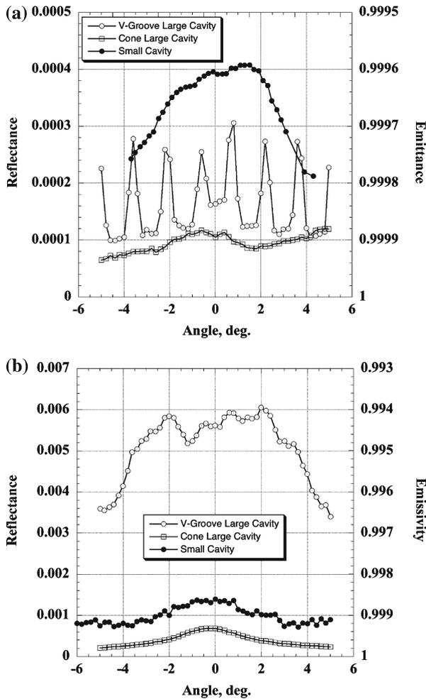
**Fig. 9** Angular dependence of effective emissivity of graphite cavities at (a)  $1.32 \mu\text{m}$  and (b)  $10.6 \mu\text{m}$
