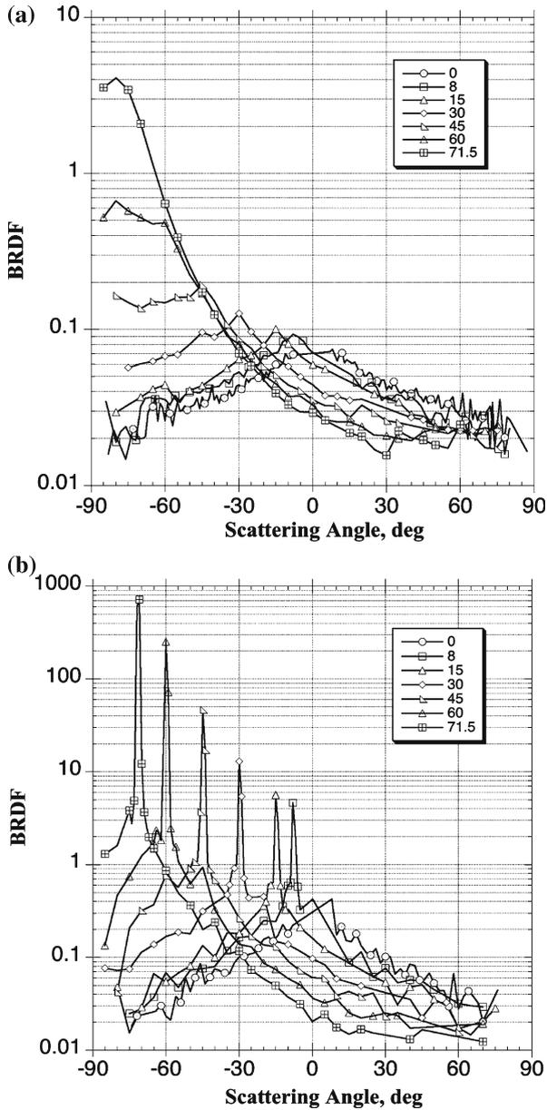
**Fig. 6** BRDF of a graphite piece of the cavity (flat back of V-groove bottom section) at (a) 1.32  $\mu\text{m}$  and (b) 10.6  $\mu\text{m}$ , for different incidence angles. Legend shows the incidence angle, in degrees, onto the sample for each curve. Scattering angle is defined with respect to the normal to the sample. No data are available within  $10^\circ$  of the incidence angle
