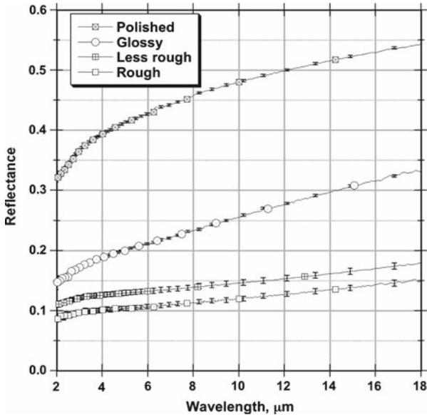
**Fig. 5** Reflectance spectra of four graphite samples with varying levels of surface roughness
